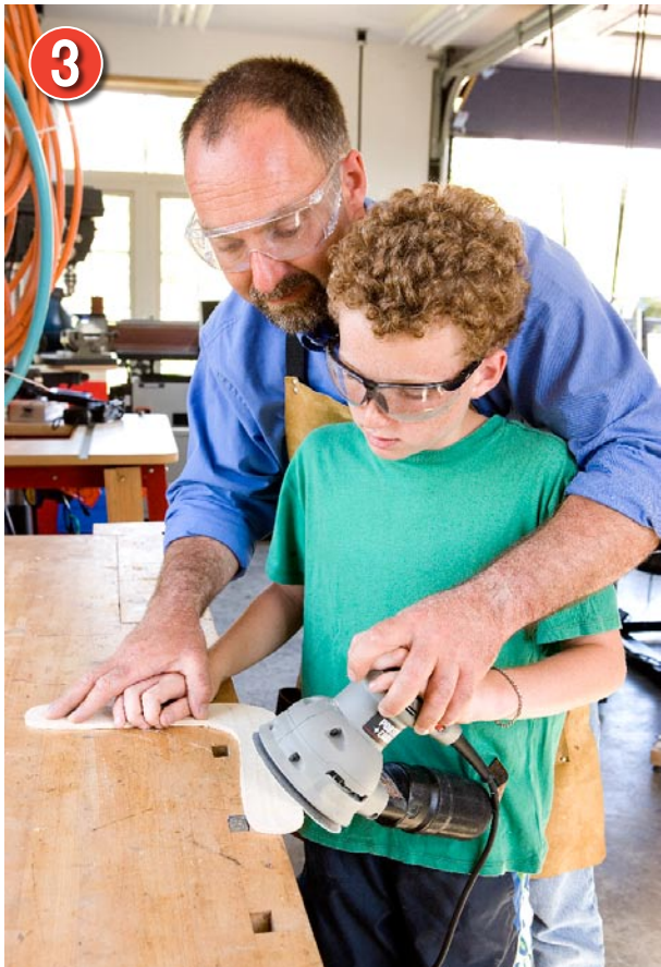
WITH A light hand, use a random-orbit sander to create the necessary curves around the leading and trailing edges
