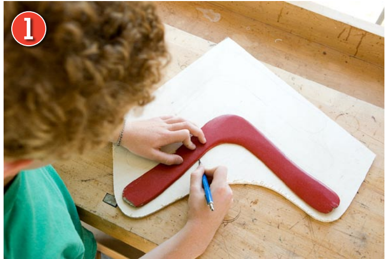
TRACE THE shape of the boomerang onto a scrap piece of plywood
