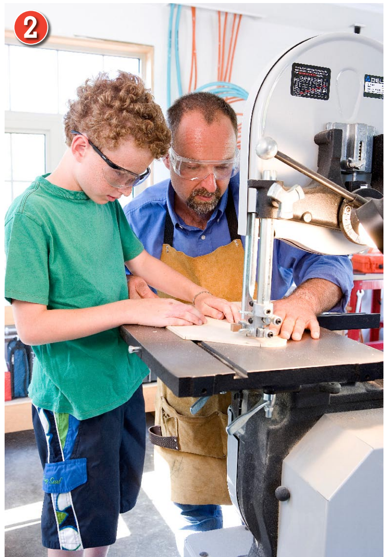
CUT OUT the shape on a bandsaw or jigsaw, staying just outside the waste line
